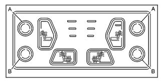
Escalade Platinum ESV vehicles will be equipped with this feature. The buttons used to control this feature are located on the instrument panel, under the radio. With the heated and cooled seats you can choose high, medium or low heat or cool settings. The seats will only operate either in the heat or cool mode; for example, you cannot cool the seat cushion while heating the seatback.
